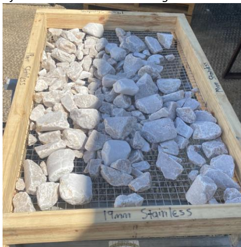
Figure 1 – Crushed, screened and scrubbed +19mm – 100mm quartz lump from Quartz Hill prepared for Sensor Based Ore Sorting Trials at TOMRA in Germany
