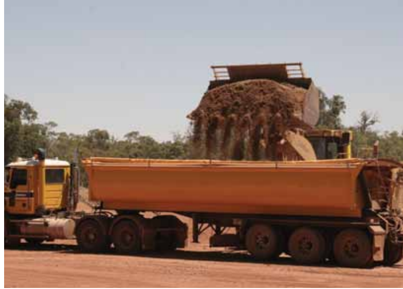
2. Bauxite ore loaded onto trucks for transport to railsiding
