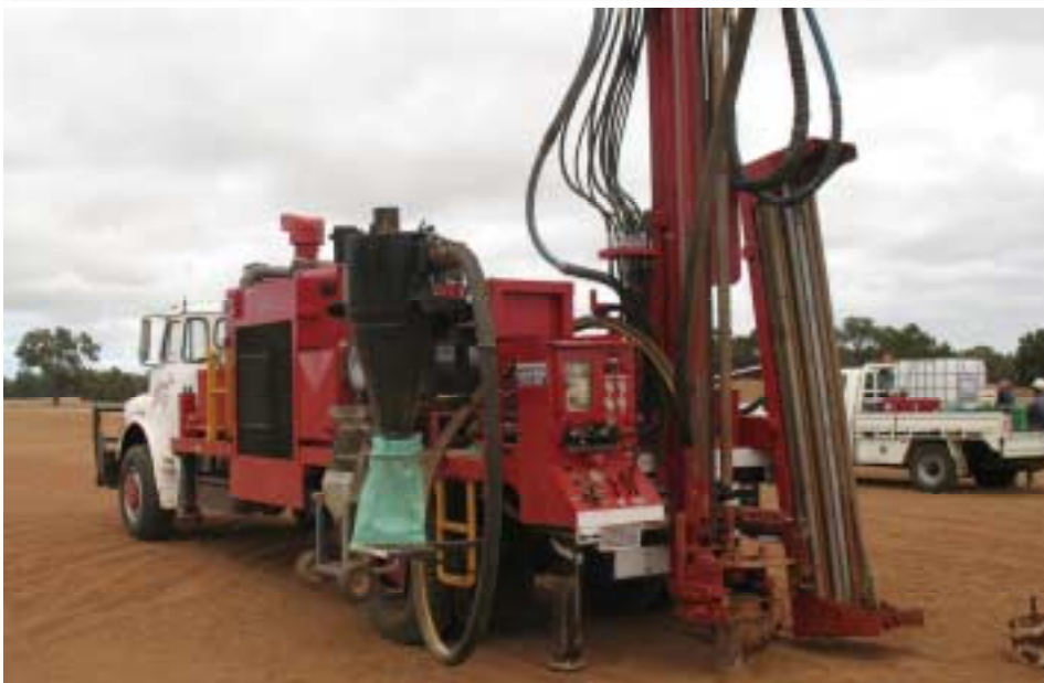
Aircore drilling rig South Darling Range project area
