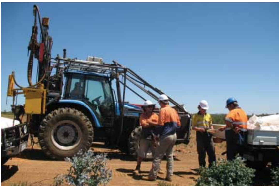
Vacuum drilling in the South Darling Range project area
