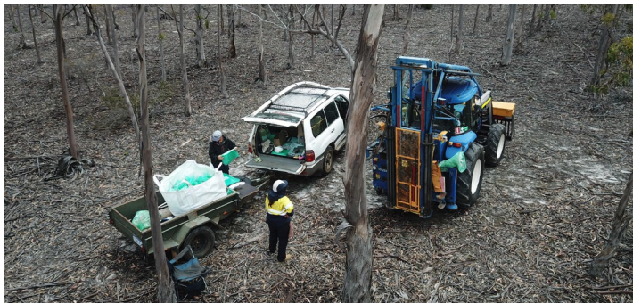
Vacuum drilling by ASQG of silica sand in a tree farm at the Albany White Sand Hill Project
