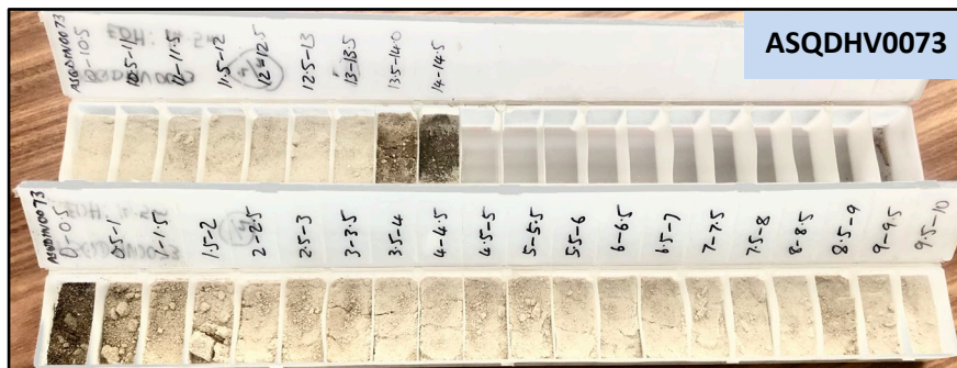
Vacuum drill hole ASQDHFV0073 sample tray showing silica sand intersection from 0.5-13.5 m
