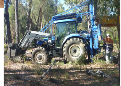
Yearlong vacuum rig used drilling programs in the Darling Range.
