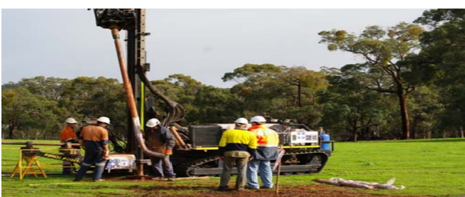
Trialling sonic drill rig at Bindoon North.
