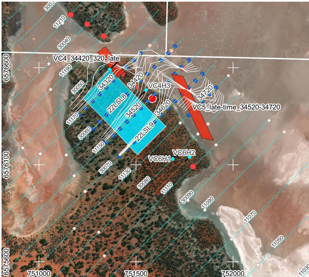
Figure 3: Modelled VC4 and VC5 FLEM conductor plates (red) with loops 22LSL8 and 22LSL9 (blue) and Bz profiles of channels 30-34 (white lines)
