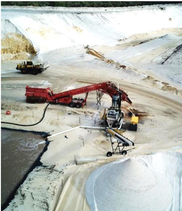
Urban's Marella Rd Silica Sand Mine with silica sand washing plant in operation
