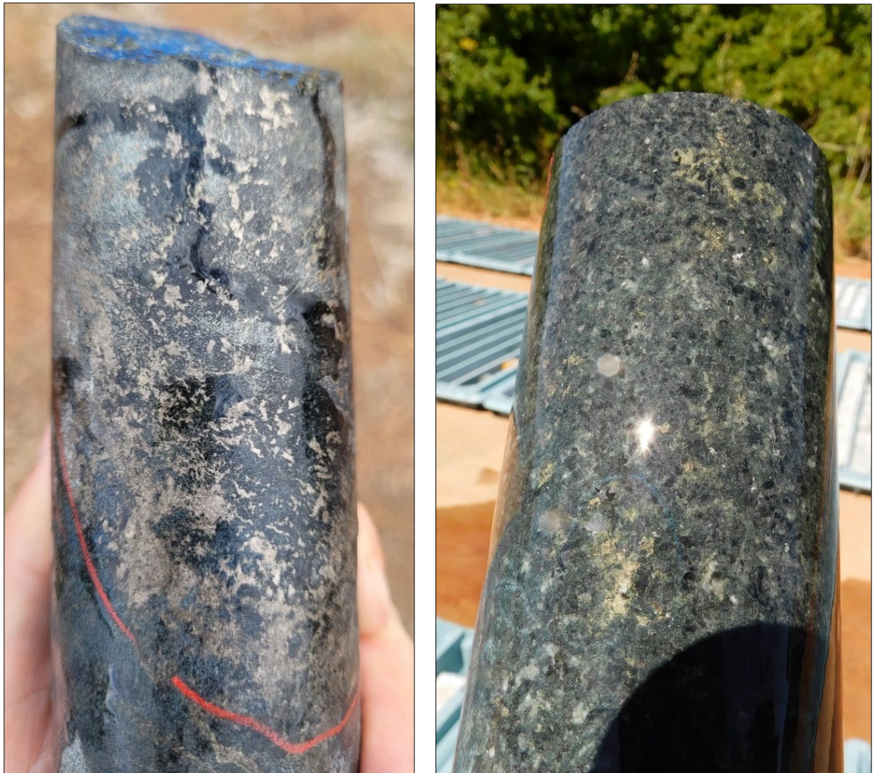
Figure 1: Matrix textured Fe-Ni-Cu sulphides within norite rock at 431.4m down-hole in Hole 2 (left) and disseminated Ni-Cu-Fe sulphides within norite rocks at 232.3m down-hole in Hole 2 (right).
