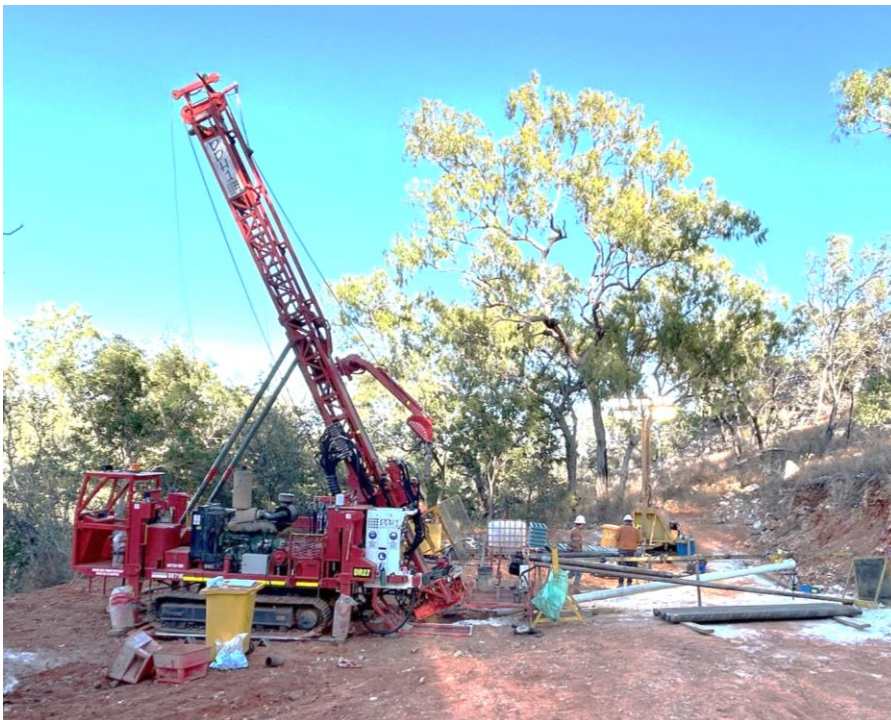
Figure 1 - Diamond Drilling commencing at Quartz Hill
